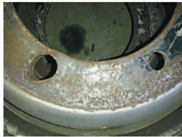
Fig. 8 — Planished holes on the disc (wheel).
