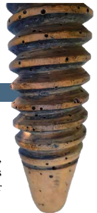
Fig. 3. Screw made of wood
