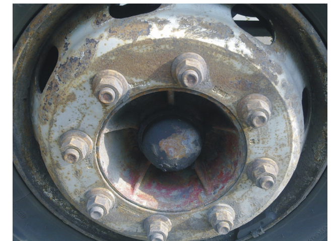
Fig. 8 Corroded bolted joints
