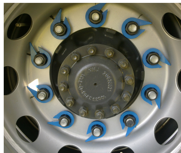
Fig. 7 Safety locks TaTrim on the wheel (a) of Renault vehicle and the stress distribution (b)
