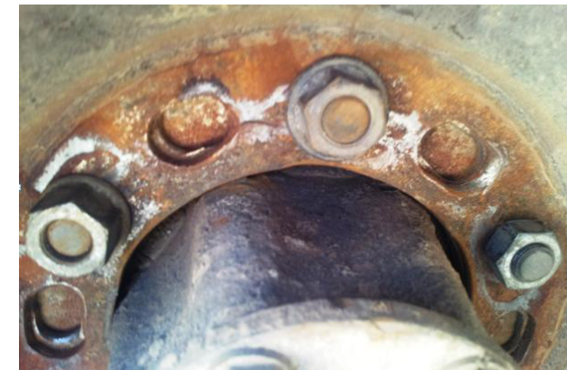
Fig. 2 The worn out original holes on the wheel disks and new holes bored amateurishly
