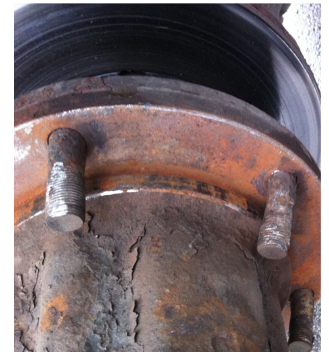
Fig. 3 The bent wheel fasteners of overloaded vehicle
